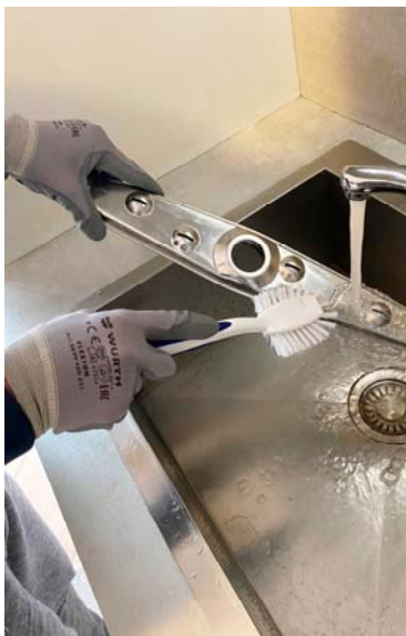
Clean the washing arm for any debris inside.
