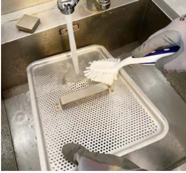
Clean the tank filters
