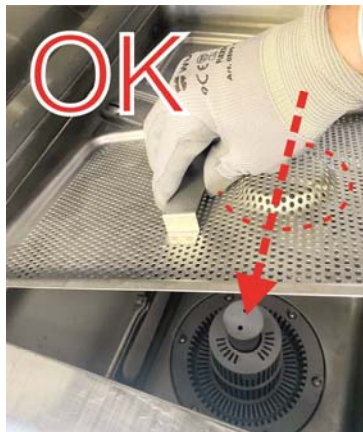
Insert the frontal tank filter. Control the right place!
