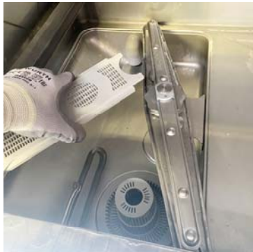
Remove the central support
