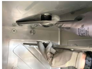
Remove the washing upper arm
