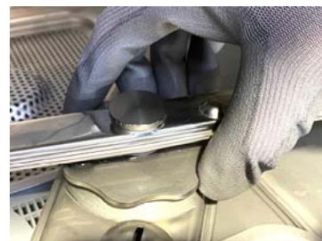
Daily disassemble the lower rinse arm by working on the „big“ ring nut
