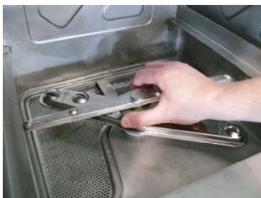
Unscrew the lower rinse arm
