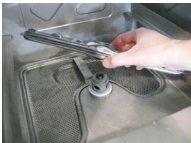
Remove the washing lower arm
